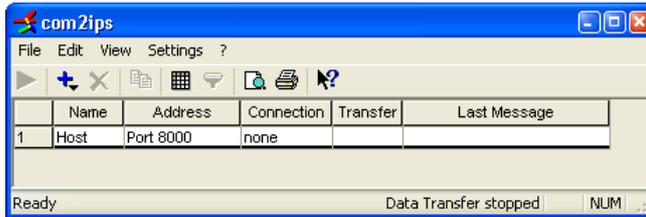
In this case, the programme will enter a TCP connection as host, with the default port 8000. The IP address is automatically the address of the computer from which com2ips has been started.
