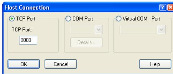
The port number for a TCP connection can be set in the dialogue “Host Connection”.
