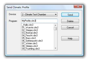
The desired target programme location for the climatic profile will be selected from this list. With new systems it will be possible to enter a programme name alternatively.
