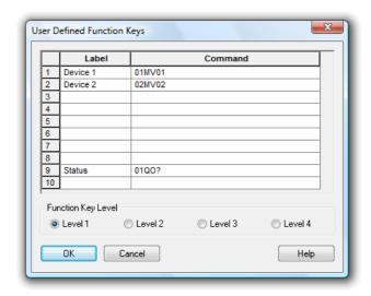
The key order in the chart is from top to bottom, as shown in the terminal window from left to right. Enter the text to be displayed by the buttons in the terminal window in the column "Label". The column "Command" contains the commands which are to be sent when the button is activated via the interface to the connected devices.
