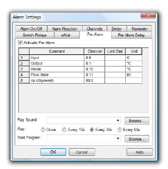
The triggering of a pre alarm can be signalled additionally by a sound or starting a program. The required entries are the same as for an alarm (cf.: Register Card "Alarm Reaction" on page 106).
