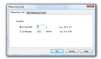
In such cases, the program will start the next cycle as soon as the hardware has processed the last cycle.
