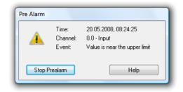
This message contains the time of the prealarm, the channel that triggered the prealarm as well as the event. The button *Acknowledge Alarm* will close the dialog, *Help* will show this text.
