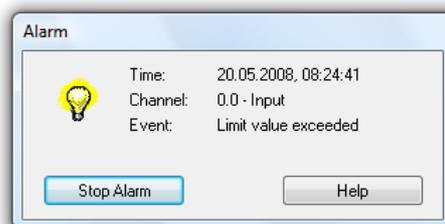
This message contains the time of the alarm, the channel that triggered the alarm as well as the event. The button *Acknowledge Alarm* will close the dialog, *Help* will show this text.
