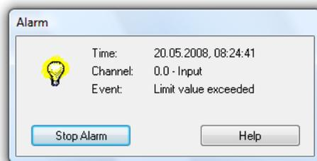
This message contains the time of the alarm, the channel that triggered the alarm as well as the event. The button *Acknowledge Alarm* will close the dialog.
